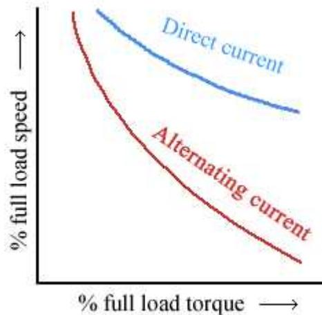
Speed/load characteristics of a universal motor is similar to that of DC series motor. The **speed of a universal motor** is low at full load and very high at no load. Usually, gears trains are used to get the required speed on required load. The speed/load characteristics are (for both AC as well as DC supply) are shown in the figure.
