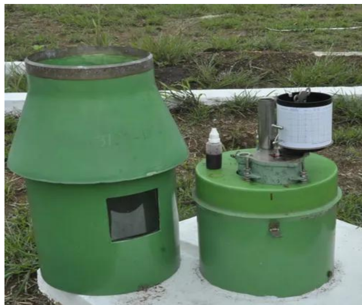
Fig 2- Recording Rain Gauge (Source: www.indiamart.com )
